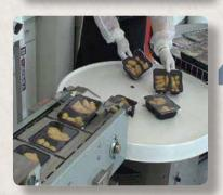
Sealed trays drop onto optional automatic Lazy Susan. Also compatible with Form Plastics optional tray filling system.
